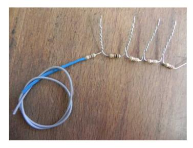
Fold the ends of the cables in a circle, and insert them in the terminals starting with the No. 1 Let the first resistor and the blue end free. (on the Pictured below, the first resistor is hidden in the blue jacket ).
