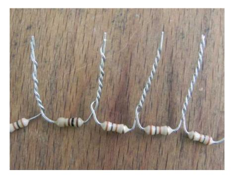
Remove all the screws and washers on the periphery of the bakelite round contact plate. Now twist the resistor soldered with the blue wire with one end of your assembly resistors :
