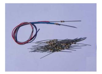
Two resistors are connected to the red and blue wires. Let them for now, and assemble the 22 resistors in this way, by twisting them with a flat nose pliers, or with your fingers.
