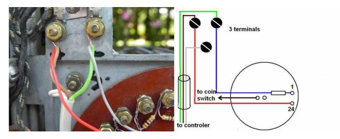
Connect the wires on the terminals as follows with the 3-conductor link cable following your wallbox model ..
