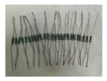
Note: resistors have no polarity and there is no particular order to meet. Let an untwisted portion of a few millimeters at the base of each resistor. If you have a soldering iron, put a bit of solder on each cable for a better grip and improved electrical contact.
