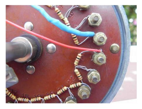
Continue that way and finish by inserting the resistor provided with the red wire on terminals 23 and 24 (red wire to terminal 24 by making a full turn around the terminal.
